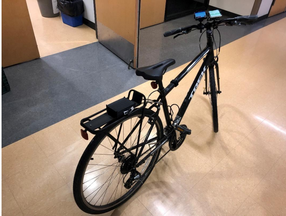
Figure 1-1: Instrumented bike with a sensor logger attached on the rear rack
